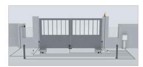
The above represented installation does not include safety devices such as safety edges. Their addition depends upon the risk assessment made on any installation in accordance with EN 12445-12453 standards.
